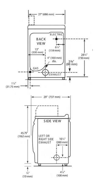
\*Use 4" (100 mm) diameter rigid aluminum or galvanized steel duct.
